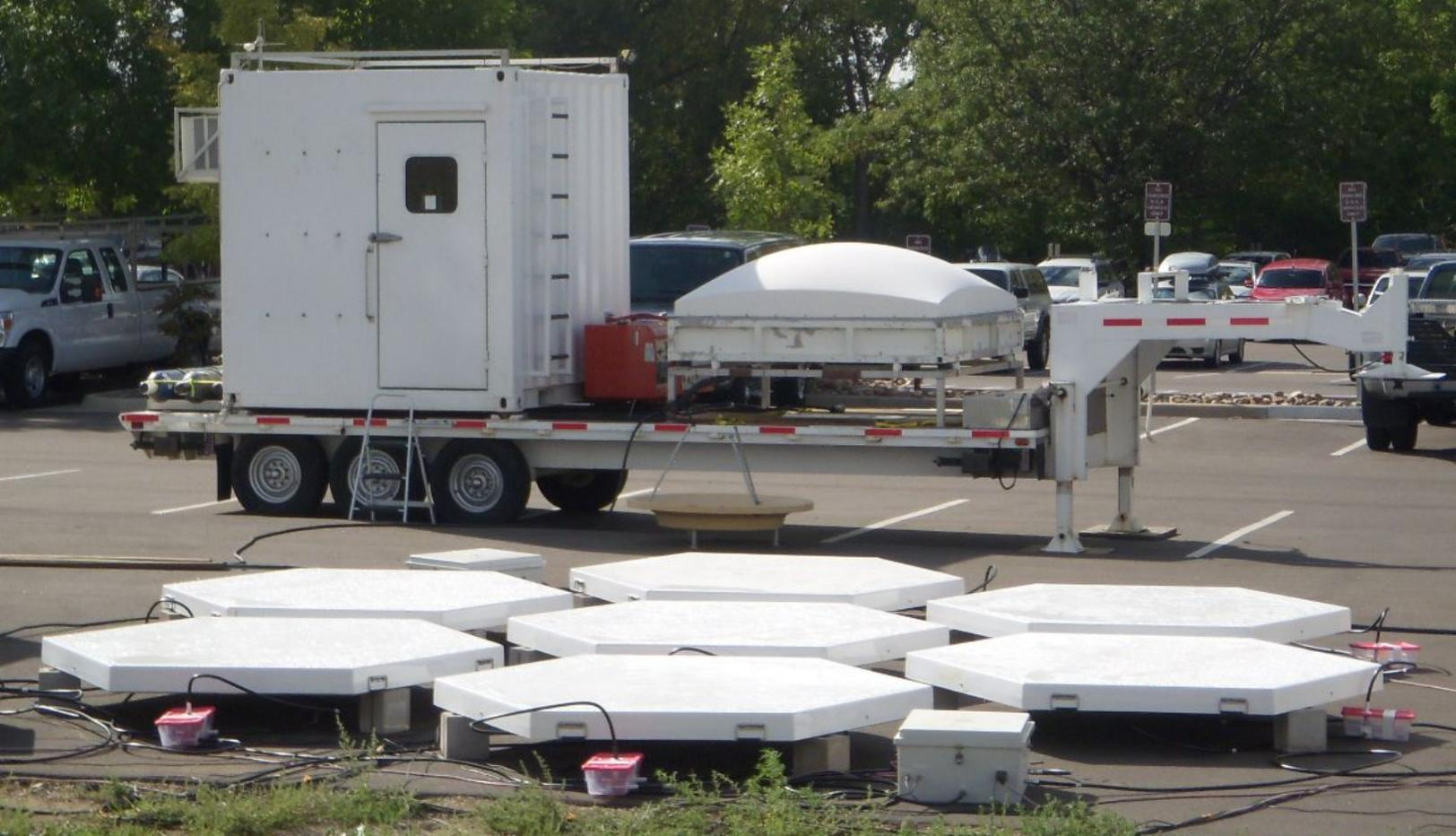
A system is typically deployed with a furnished trailer, which transports the equipment to a field site and then acts as office space and shelter for computers and other equipment.
