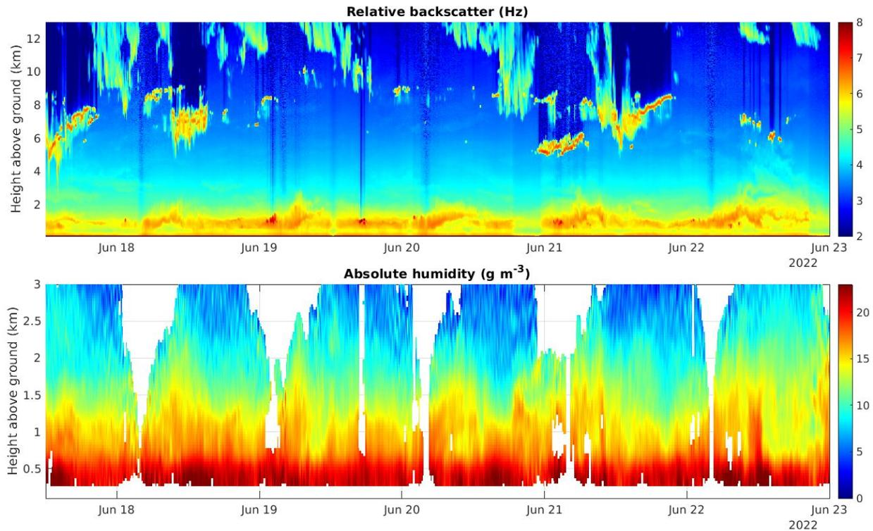
*MPD data collected in June 2022 during the Taiwan-based PRECIP field program. The top panel shows relative backscatter; the bottom panel shows absolute humidity.*
