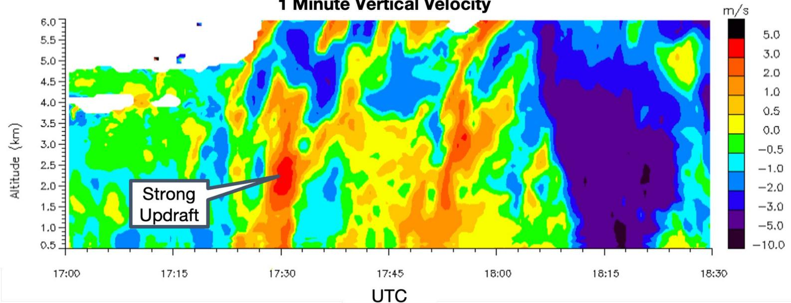
*The data plot shows 1 min vertical velocity data from the NCAR 449 MHz wind profiler (3 panels) during the CHEESEHEAD campaign in summer 2016.*
