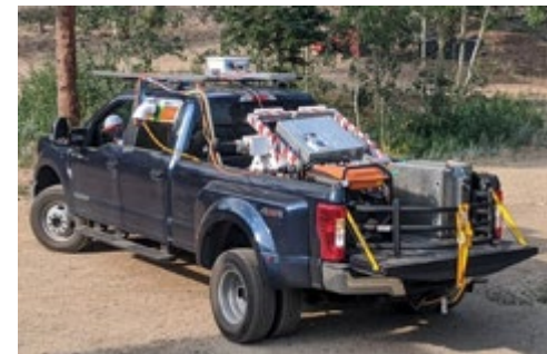
Vertical velocity and horizontal wind profiles from truck mounted mobile lidar
