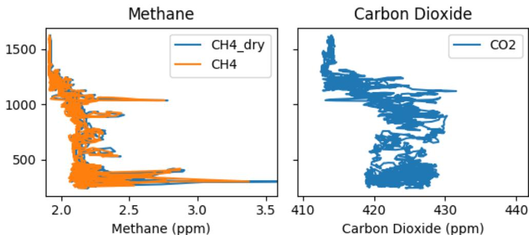
Figure 23: Carbon dioxide and methane mole fractions vs. altitude collected on spiral flights around the Bailey coal mine in southwestern Pennsylvania. Flight time is midday. Figure courtesy D. Wesloh.
