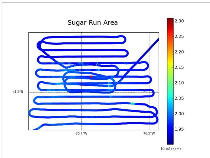
Figure 25: Methane mole fractions observed during a gridded flight over the Sugar Run watershed, east of Williamsport, Pennsylvania. Gridded flights were conducted at approximately 300 meters AGL, and at midday. A red star indicates the Sugar Run watershed.
