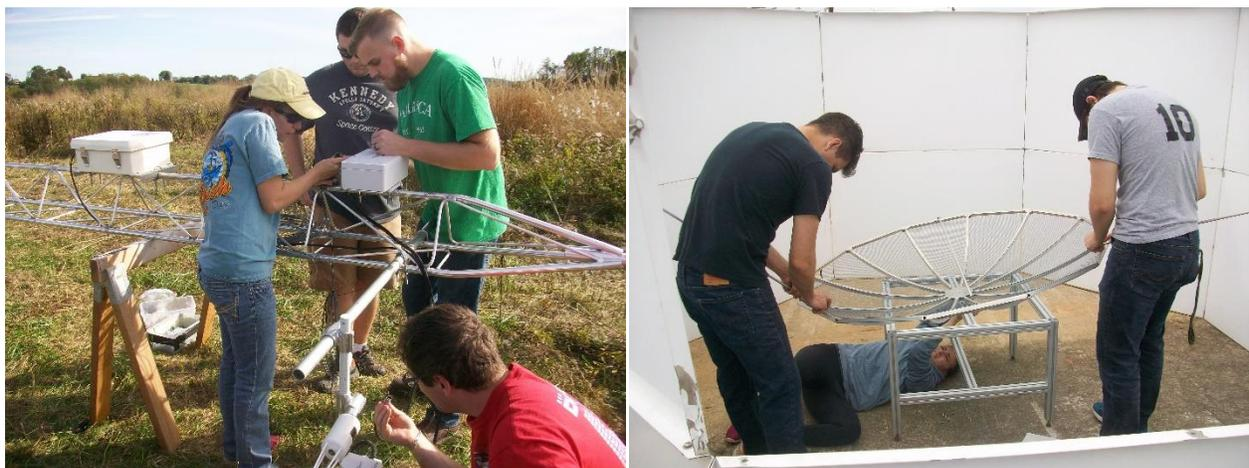
Figure 37: Students attach instruments to the 10 m flux tower (left) and anchor the RASS dish on the SoDAR (right). In addition, students were required to learn the theory of operation of all the sensors on each platform.
