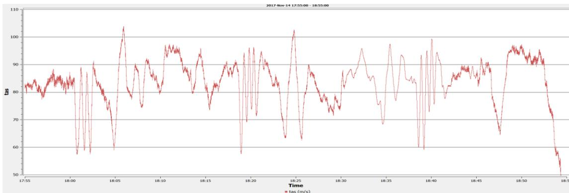
Figure 31: King Air aircraft true airspeed measurements. Note the three periods of regular variation that represent a series of maneuvers to vary airspeed.
