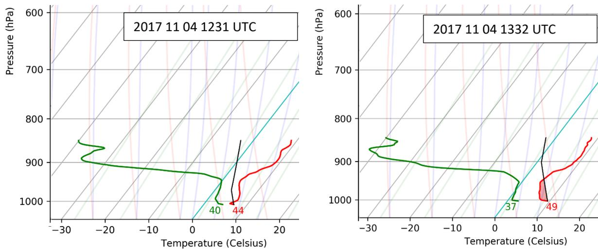
Figure 13: Vertical profiles of temperature (red) and dew-point temperature (green) for Sharpsburg, MD at 1231 UTC (left) and Waynesboro, PA at 1332 UTC (right) during a cold-air damming event (RF01)
