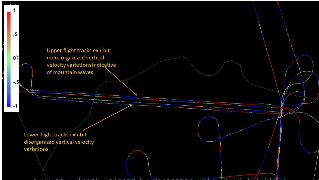
Figure 16: Flight tracks colored with vertical velocities. The four east-west stacks are indicative of regular mountain wave undulations residing on top of a turbulent boundary layer during RF07.
