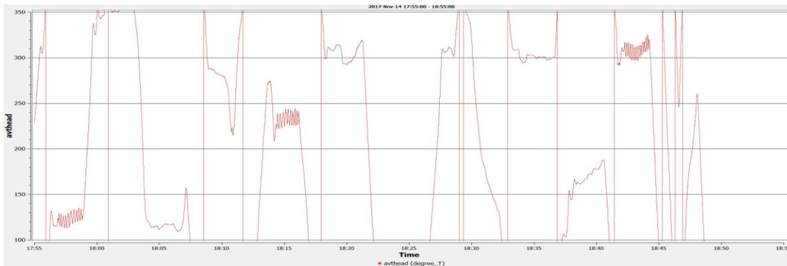
Figure 30: King Air aircraft true aircraft heading measurements. Note the three periods of regular variation that represent a series of maneuvers to vary yaw via the rudder.
