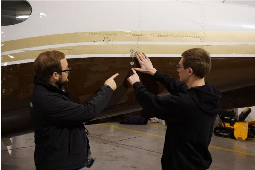
Figure 29: Two MU students point out the location of the static pressure port in the aft section of the fuselage of the King Air.
