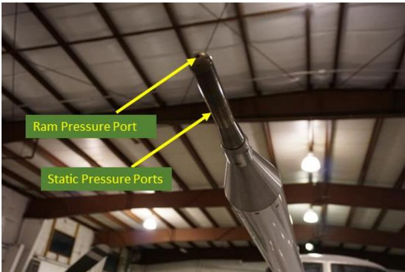
Figure 30: Close-up of the tip of the gust probe of the UWKA showing the ports used to measure ram (dynamic) and static pressure. Bernoulli's Principle for a compressible fluid is used to determine the true air speed.
