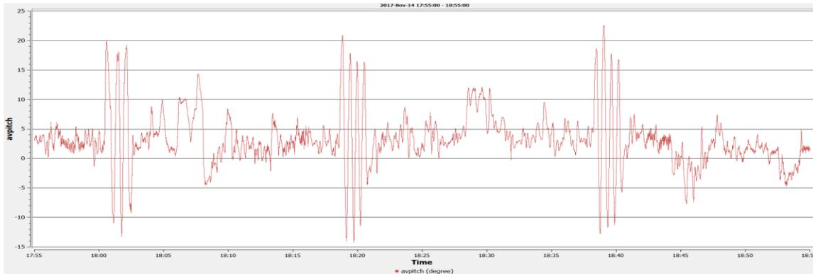
Figure 34: King Air aircraft pitch measurements. Note the three periods of regular variation that represent a series of porpoising maneuvers.
