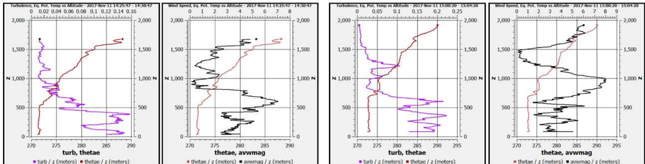
Figure 19: Vertical profiles from Cumberland, MD (left two) and Bendigo, PA (right two) on 11 NOV 2017 showing equivalent potential temperature (red), turbulence intensity (magenta), and wind speed (black) during an Appalachian cold-pool event.
