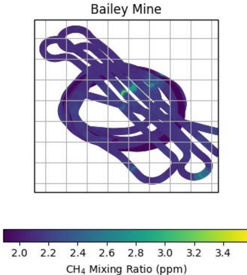
Figure 22: Methane mole fractions in a small circle (3 km radius) around the Bailey coal mine in southwestern Pennsylvania during SEAR-MAR RF06 on 9 NOV 2017. Most of the data are within the atmospheric boundary layer. Flight time is midday. Figure courtesy D. Wesloh.
