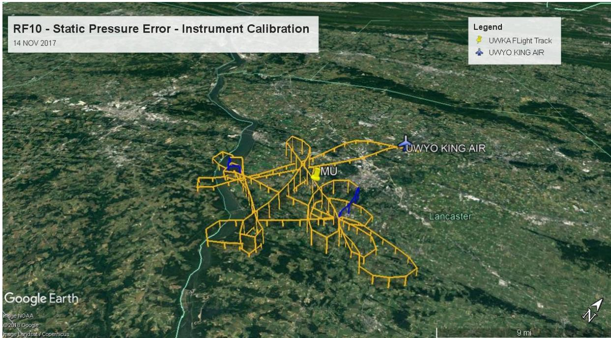
Figure 31: Flight pattern used for the determination of the aircraft static pressure error. The pattern was designed to maximize the variation in aircraft parameters (pitch, roll, yaw, airspeed, etc.) and to gather a sufficiently long data set to provide a statistically robust algorithm with which to estimate the error in static pressure measured at the static ports.
