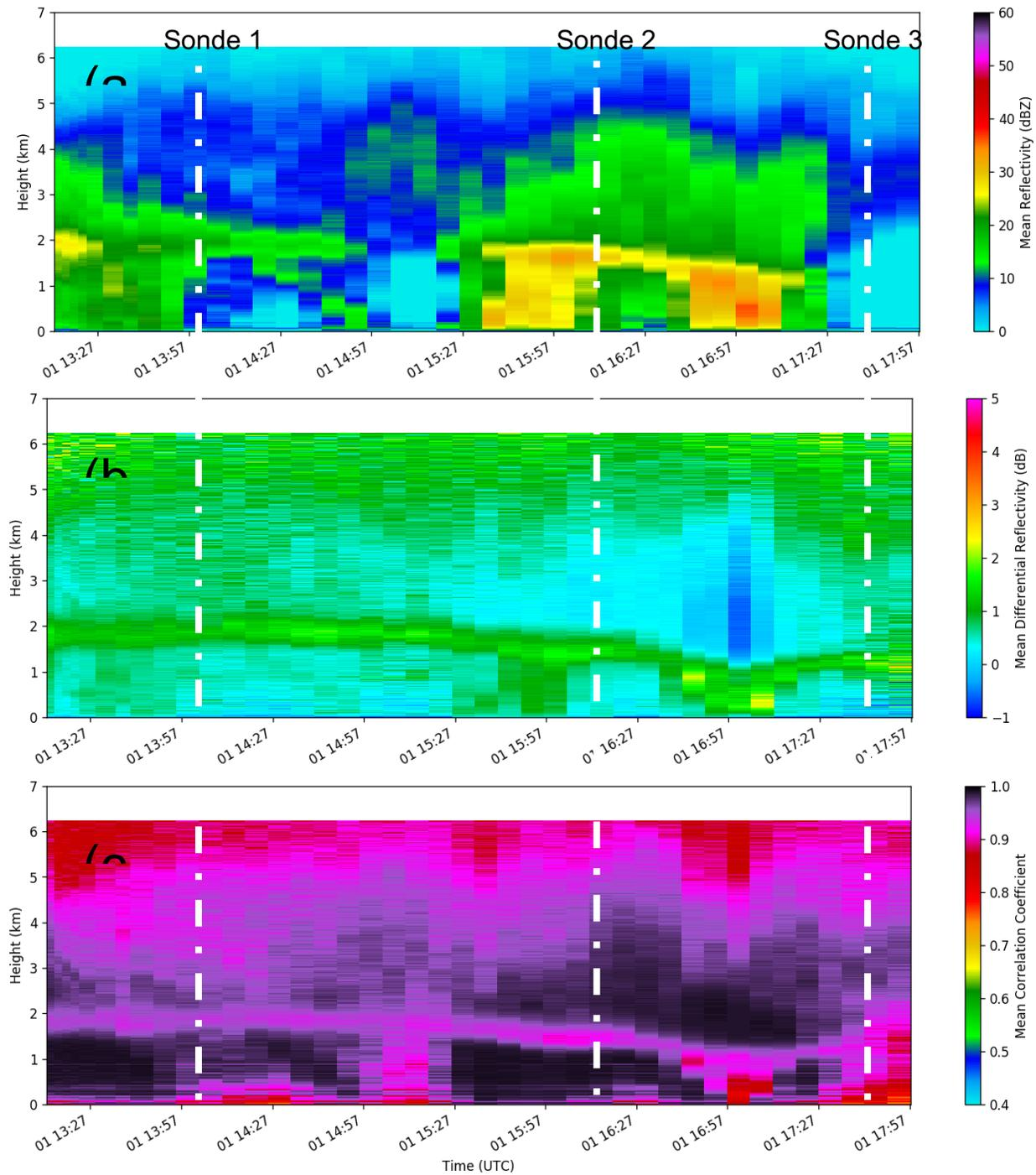
Fig. 7. QVPs of DOW7 observations of (a) reflectivity (in dBZ), (b) ZDR (in dB), and correlation coefficient (unitless) for IOP1. White, vertical dot-dash lines indicate the times of sonde launches from campus (Fig. 6). Images courtesy P. Saunders.
