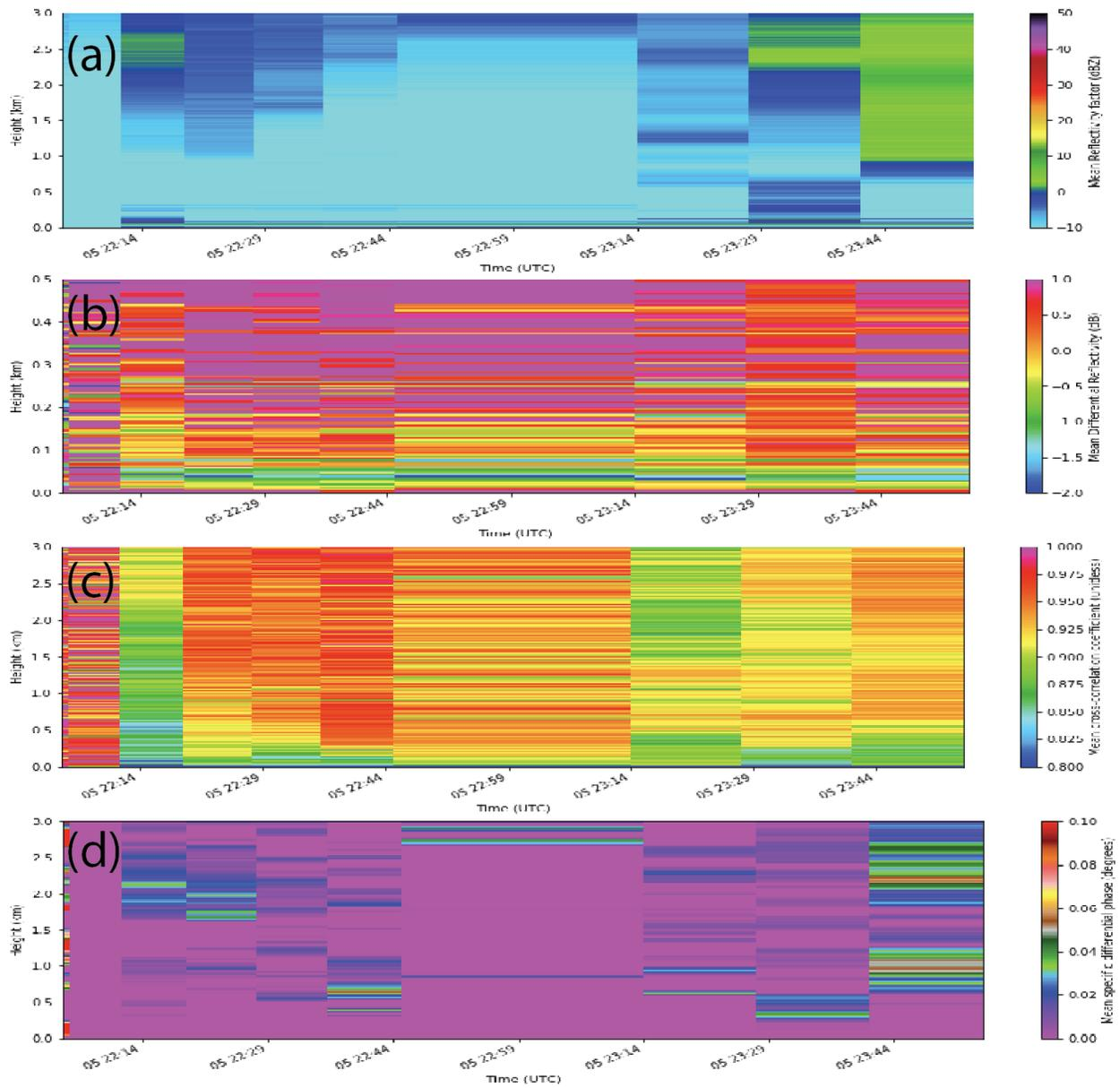
Fig. 12. QVPs of DOW7 observations of (a) reflectivity (in dBZ), (b) ZDR (in dB), (c) correlation coefficient (unitless), and (d) specific differential phase for a portion of IOP2. Image courtesy of J. Chen.
