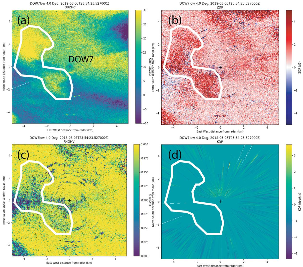
Fig. 13: PPI displays of DOW7 (a) reflectivity (in dBZ), (b) ZDR (in dB), (c) correlation coefficient (unitless), and (d) specific differential phase (in  $\text{deg km}^{-1}$ ) at 2354 UTC on 5 March 2018 at an elevation angle of  $4.0^\circ$ . The view is confined to a 5 km x 5 km box centered on DOW7 (whose location is marked by a black cross). A possible refreezing signature is outlined in white.
