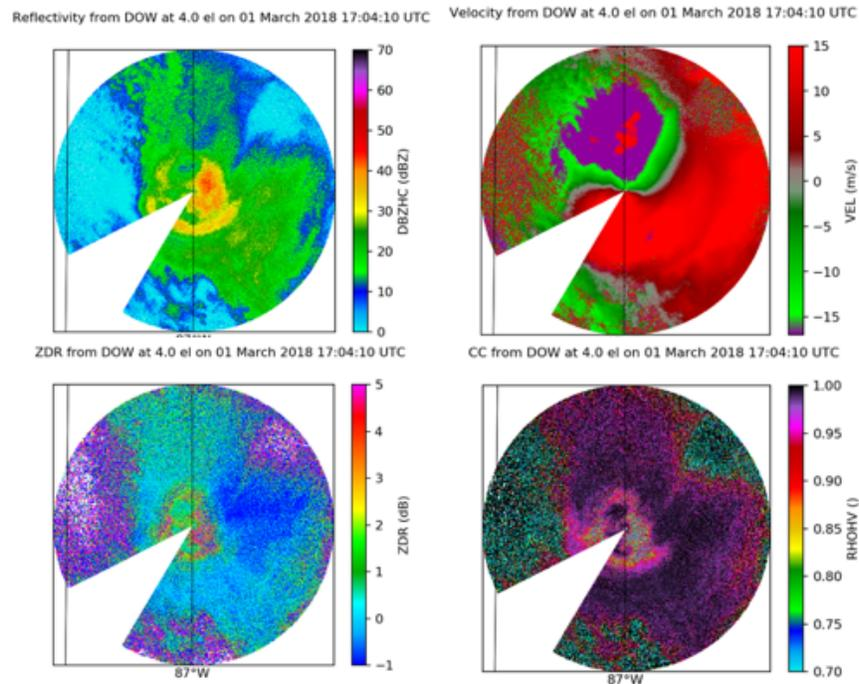
Fig. 8. (clockwise from top left) PPI displays of DOW7 reflectivity (in dBZ), Doppler velocity (in  $\text{m s}^{-1}$ ), correlation coefficient (unitless), and ZDR (in dB) at an elevation angle of  $4.0^\circ$  at 1704 UTC.
