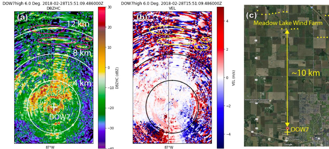
Fig. 3. (a) Reflectivity (in dBZ) and (b) Doppler radial velocity (in  $\text{m s}^{-1}$ ) measured by DOW7 at  $6.0^\circ$  elevation during a clutter survey at ACRE on 28 February 2018. (c) Satellite imagery (courtesy Google Maps) of the same area, with the locations of wind turbines in the Meadow Lake Wind Farm plotted as yellow dots. Corresponding echoes are circled in magenta in panel (a) and yellow in panel (b).
