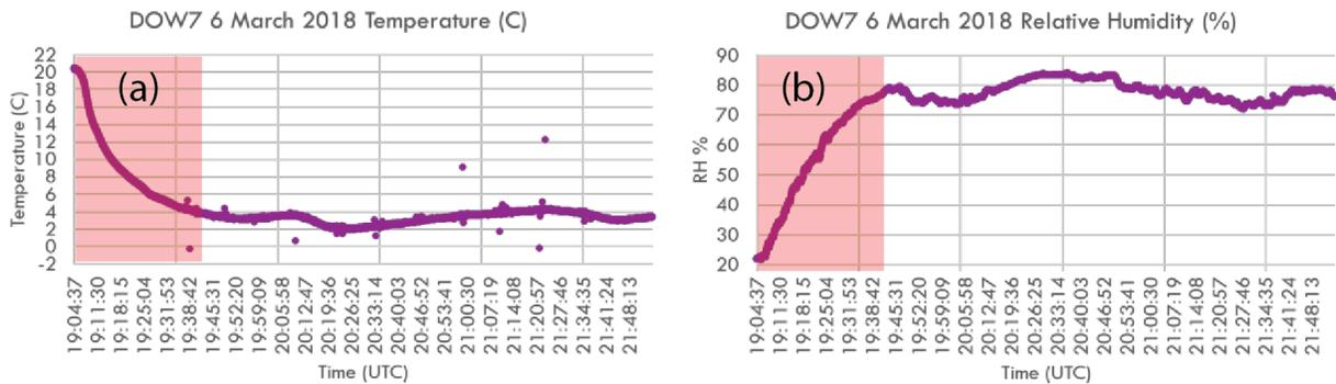
Fig. 15. Air temperature (in deg C) and relative humidity (in percent) observed by the DOW pod during IOP3. The red shaded area denotes when the DOW was still equilibrating to the outdoor conditions after departing the garage (Fig. 2) and are not representative of the environmental conditions at ACRE. Base image courtesy of A. LaFleur.
