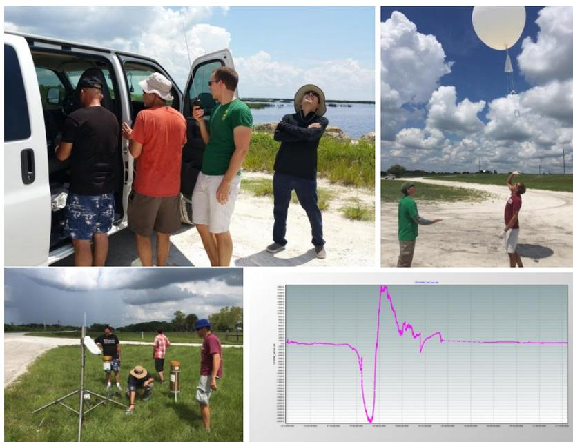
**Fig. 9.** TOP Left: Graduate student Brett Dean, Dr. Lazarus, graduate student Bryan Holman (holding the iMet radiosonde receiver) and Dr. Ray gazing upwards at the ascending balloon. TOP RIGHT: Sophomore Alex Robertson and graduate student Jeff Colvin watch as the balloon is released. BOTTOM: Setting up the field meter as the storm approaches (left) and field meter data as storm passed overhead (right).
