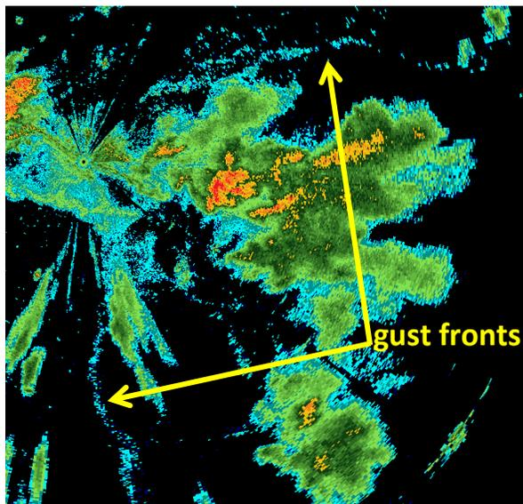
**Fig. 11.** DOW-7 reflectivity (1 degree tilt) valid 1840 UTC 6 September 2015. The radar was parked on a levy along the north shore of Lake Okeechobee. Several gust front boundaries are visible in this image (courtesy of graduate student Bryan Holman).
