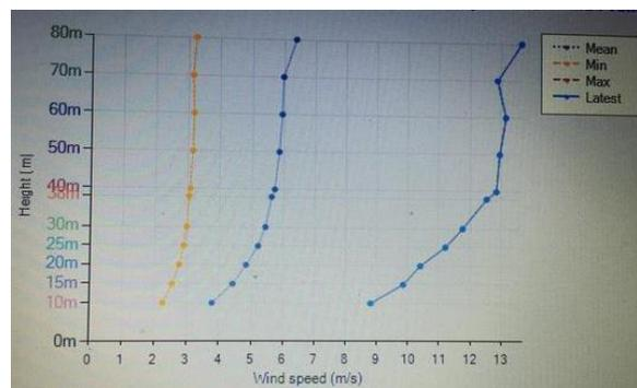
**Fig. 12.** Lidar wind profiles (min, max, and mean in m/s) from 8 September 2015 gust front passage in Melbourne.
