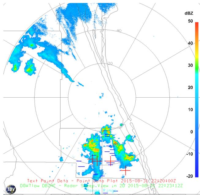
**Fig. 5.** DOW-7 reflectivity (dBZ, 3 degree tilt) valid 2223 UTC 31 August 2015 (color filled). Also shown are the 5 min window of NLDN cloud-to-ground lightning locations (with polarity).
