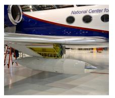
NCAR HIAPER Cloud Radar (HCR) can be mounted to the underside of the wing of the NSF/NCAR HIAPER research aircraft (a modified Gulfstream V jet) and delivers high quality observations of winds, precipitation and other particles. It was designed and manufactured by a collaborative team of mechanical, electrical, aerospace, and software engineers; research scientists; and instrument makers from EOL.
