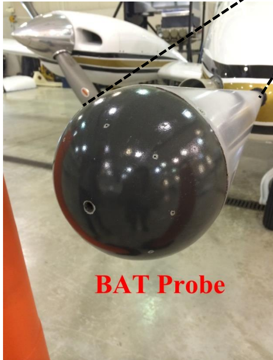
BAT: Best Air Turbulence probe up to 50 Hz turbulence wind
