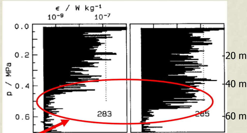
Dissipation varies by a factor of  $\sim 100$  between the two casts, for no obvious reason other than the intermittency of turbulence
