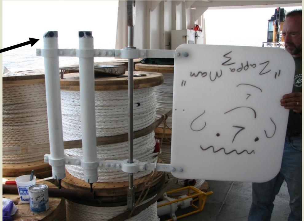
A single horizontal beam measures a  $\sim 1.5$ -m profile with  $\sim 3$ -cm resolution, which can be used for inertial-subrange estimates of dissipation (i.e., fitting a  $-5/3$  power law to velocity spectra)
