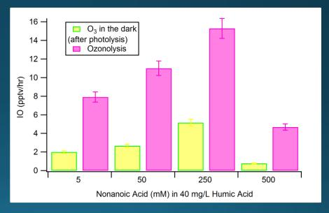
Photosensitizers, in this case humic acid, activates iodine which is later reacted with gas-phase ozone to produce IO.
