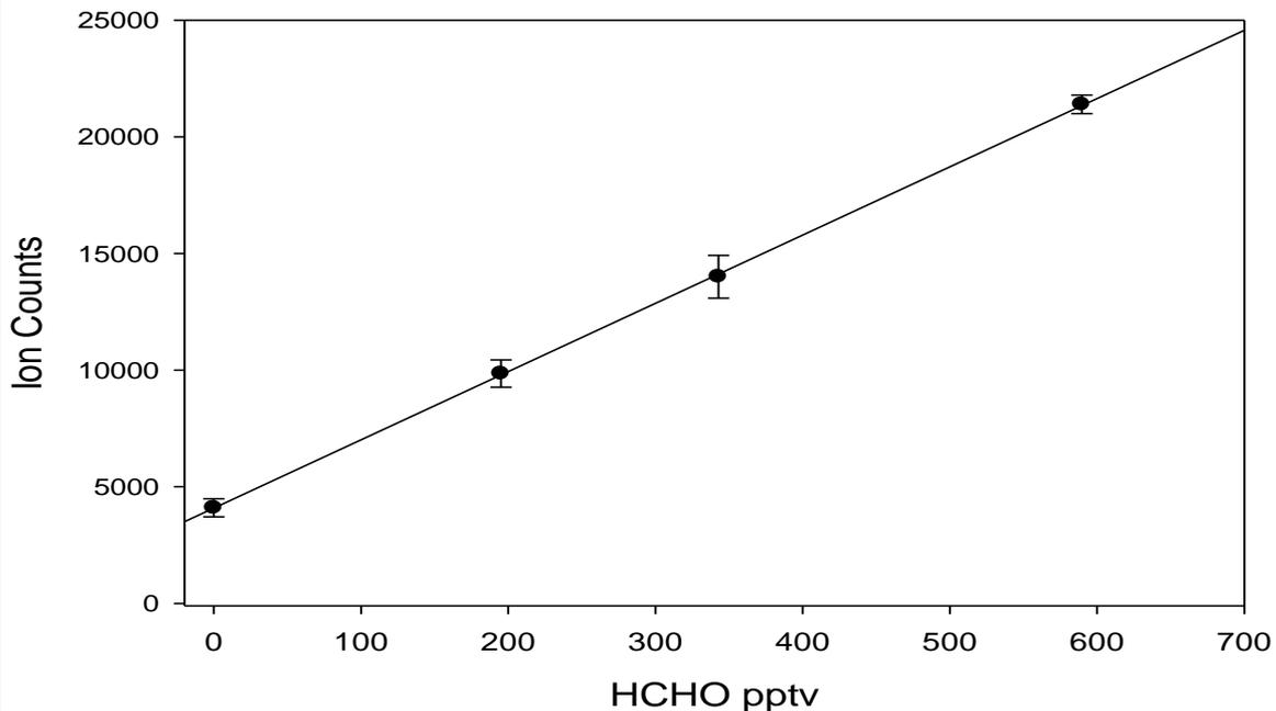
Calibration curve for the TOGA low concentration formaldehyde study. Five measurements were obtained for each data point using formaldehyde standards introduced to TOGA. The standards were generated using the permeation system described in Figure 2 coupled to the dilution apparatus described in Figure 4.
