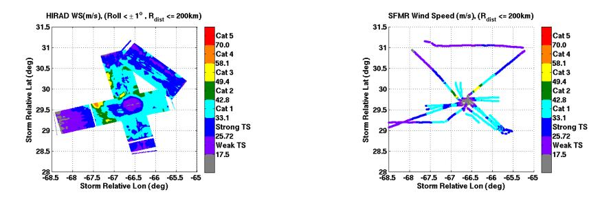
HIRAD paints more complete picture of the storm with only two passes from WB-57, compared to nadir-viewing SFMR with several passes on low-altitude recon aircraft
