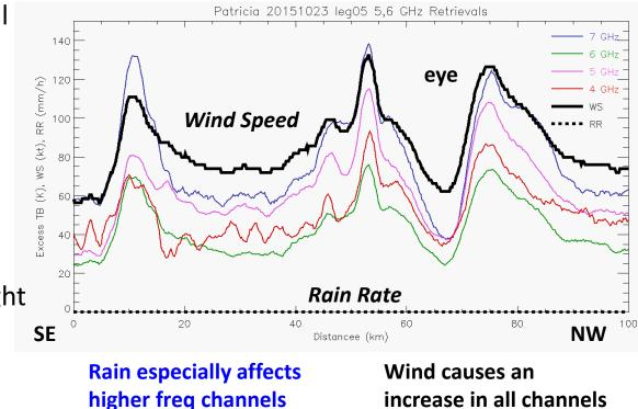
6 GHz channel is biased low in this Hurricane Patricia example. 2-channel retrieval using 5 & 6 GHz interprets everything as wind, with no rain, because 6 GHz is too low
