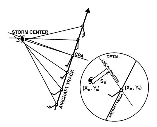
Consider these seven vector wind directions are to be extracted at specific elevations from seven HDSS soundings deployed from the NASA WB57 aircraft overflying the tropical cyclone center at 60,000 ft at a speed of 400 mph
