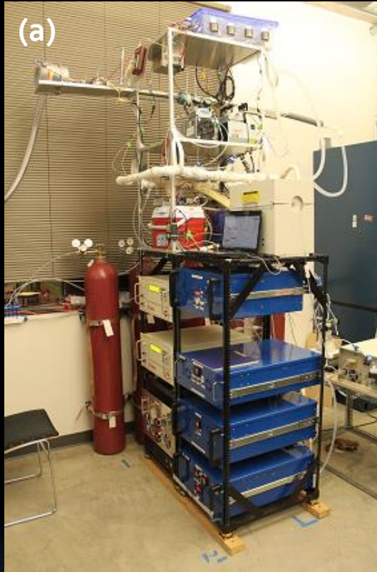
(a) Manifold/spiking system; (b) measured vs. expected manifold HgBr 2 concentrations
