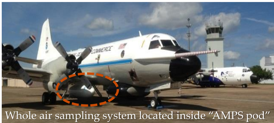
On-board sampling system designed by NCAR
