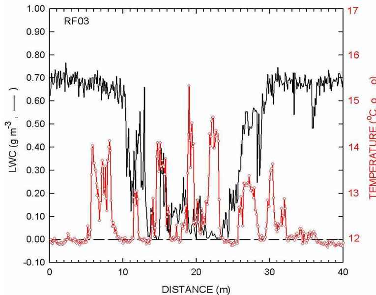
**Figure 1** - 1000-Hz (10-cm horizontal resolution) measurements of LWC with the PVM (Particulate Volume Monitor) and the UFT (ultra-fast temperature probe for in-cloud and out of cloud measurements; Haman et al, 2001) made in a mixing episode near Sc cloud top from the C-130 aircraft during DYCOMS-II. A ~6-m separation on the aircraft wing of the probes prevents proper correlation of the data.
