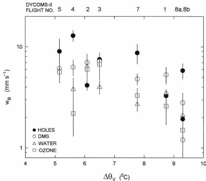
**Figure 2** - Comparison of  $w_e$  for four independent measurements on the NSF C-130 during DYCOMS II as a function of the buoyancy jump ( $\Delta\theta_v$ ) at cloud top. Solid data are for conditional sampling of “cloud holes”(Gerber et al, 2005), and hollow data are for the “flux-jump” method using DMS, total water, and ozone (Faloona et al, 2005).
