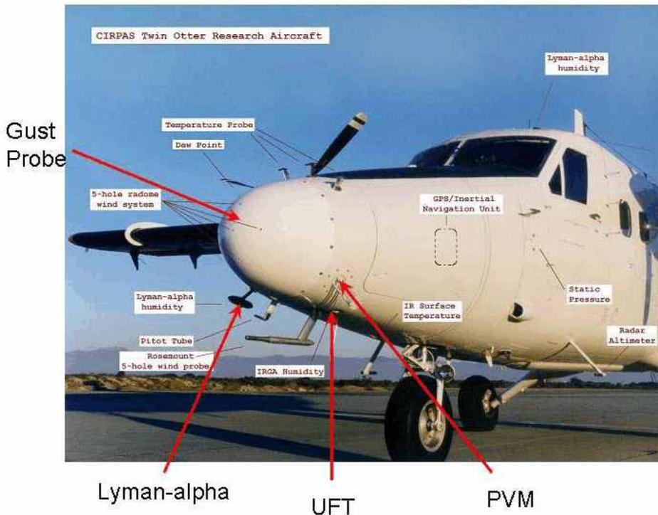
large nose compartment for mounting additional sensors. Figure 3 shows the atmospheric probes clustered around the nose ring slightly aft of the gust-probe system (some other sensors are also shown). Details on a similar radome wind system (gust probe) can be found in Khelif et al (1999).
