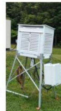
(Above) CFH and RS92 preparation and launch. (Right) surface reference system for pre-launch sonde characterization
