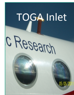
TOGA inlet on GV
