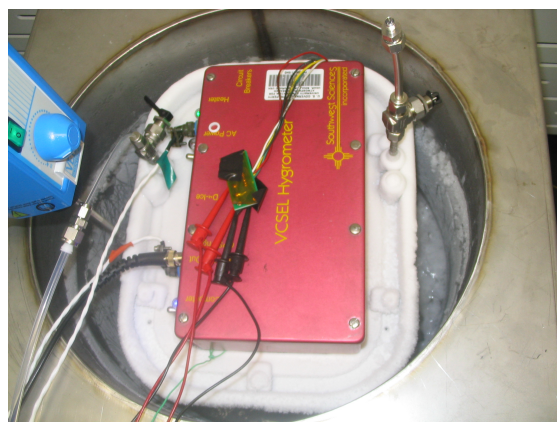
d) VCSEL isolated in cold bath
