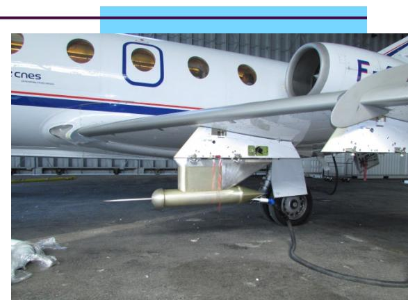
*Isokinetic TWC Evaporator on Falcon-20, unique new instrument for high IWC measurement*
