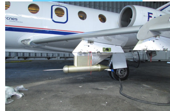
Isokinetic TWC Evaporator on Falcon-20, unique new instrument for high IWC measurement
