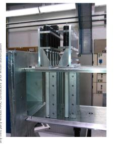
**DGA -** Collection of supercooled droplets produced by the spray bars on rotating cylinders and scratching of ice layer by saw blades
