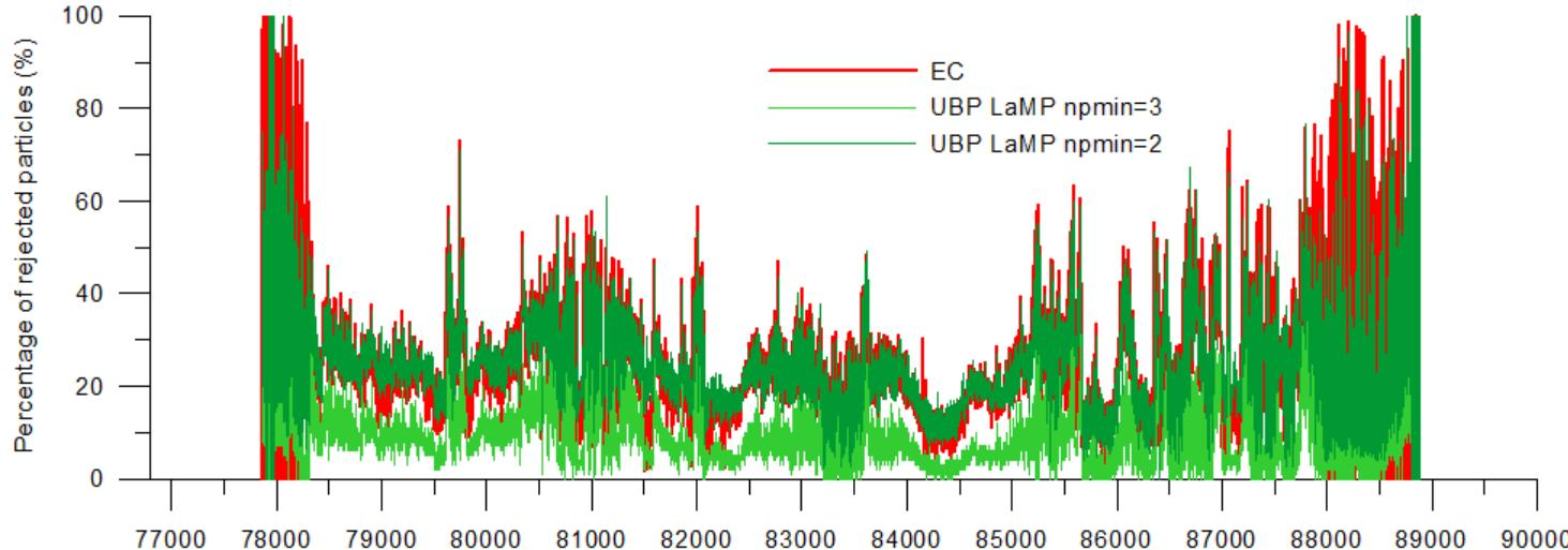
Changing the threshold from 2 particles to 3 particles causes a major reduction in the number of rejected particles.
