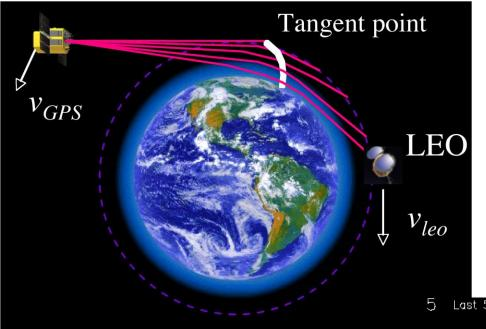
The LEO tracks the GPS phase while the signal is occulted to determine the Doppler
