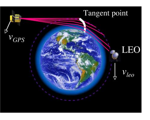
The LEO tracks the GPS phase while the signal is occulted to determine the Doppler
