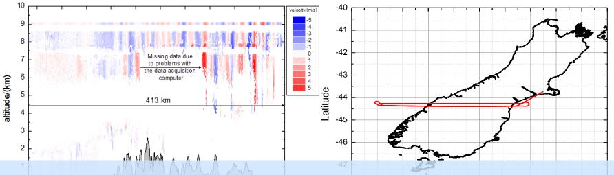
It has to be verified if "nadir" pointing was set correctly during flight (especially perpendicular to flight direction). Different legs and wind vector measurement might be used for correction.
