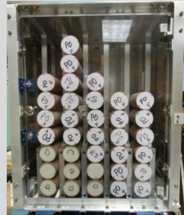
Sonde storage in launcher
