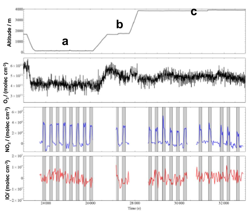
The left graph shows flight altitude, ozone number density as well as retrieved NO<sub>2</sub> and IO number densities during the three SLRs at different altitudes during flight B837.
