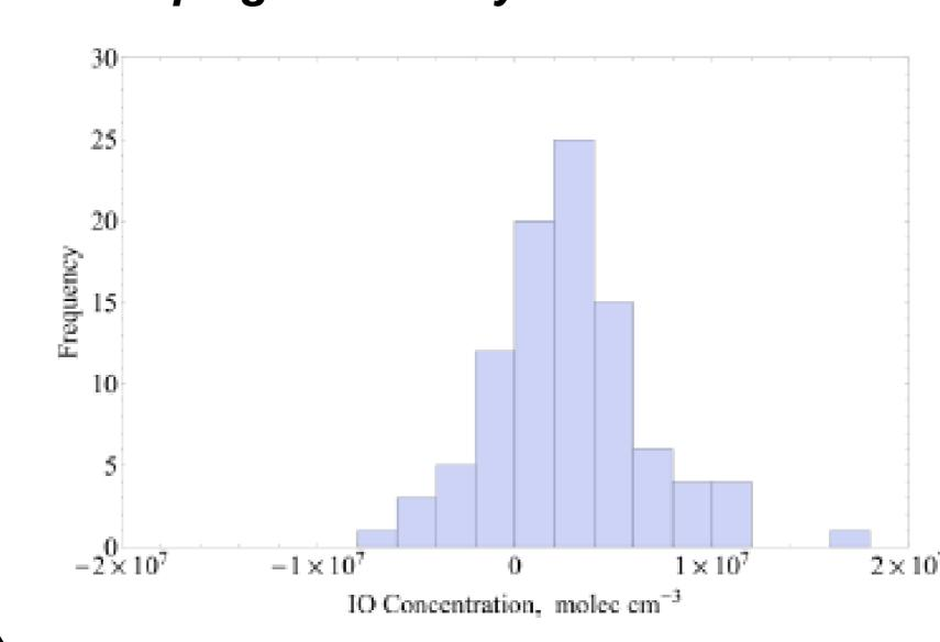
Left shows the histogram of retrieved IO (referenced to the baseline from NO titration) from 97 level runs during the entire CAST campaign. The distribution seems to skew towards positive values of IO at sub-ppt level. Further analysis of altitude dependence (not shown) however shows no clear trend.
