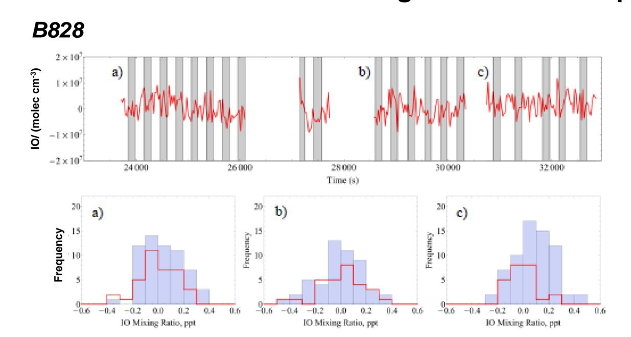
Above shows the time series of retrieved mixing ratios of IO at three different SLRs during flight B828 (also see left), together with the histogram of retrieved IO when NO titration was off (blue columns) and that of IO when NO titration was on (overlaid red lines). Comparison of the two appears to show positive bias of < 0.2 ppt, yet with little altitude dependence.
