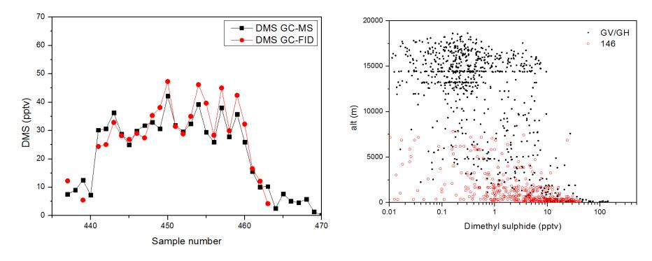
DMS well characterised between CAST WAS instruments • Compares well in vertical profile to AWAS (GV/GH)
