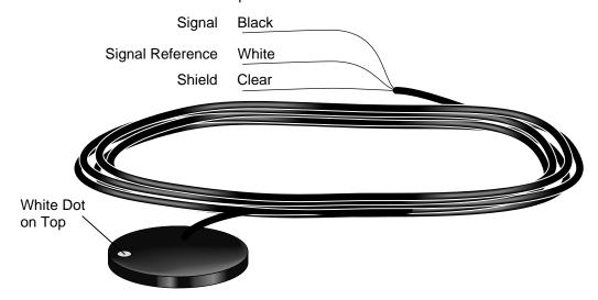
FIGURE 2. HFT3 Plate to Datalogger Connections
