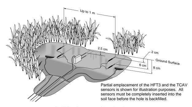
FIGURE 1. Placement of Heat Flux Plates
