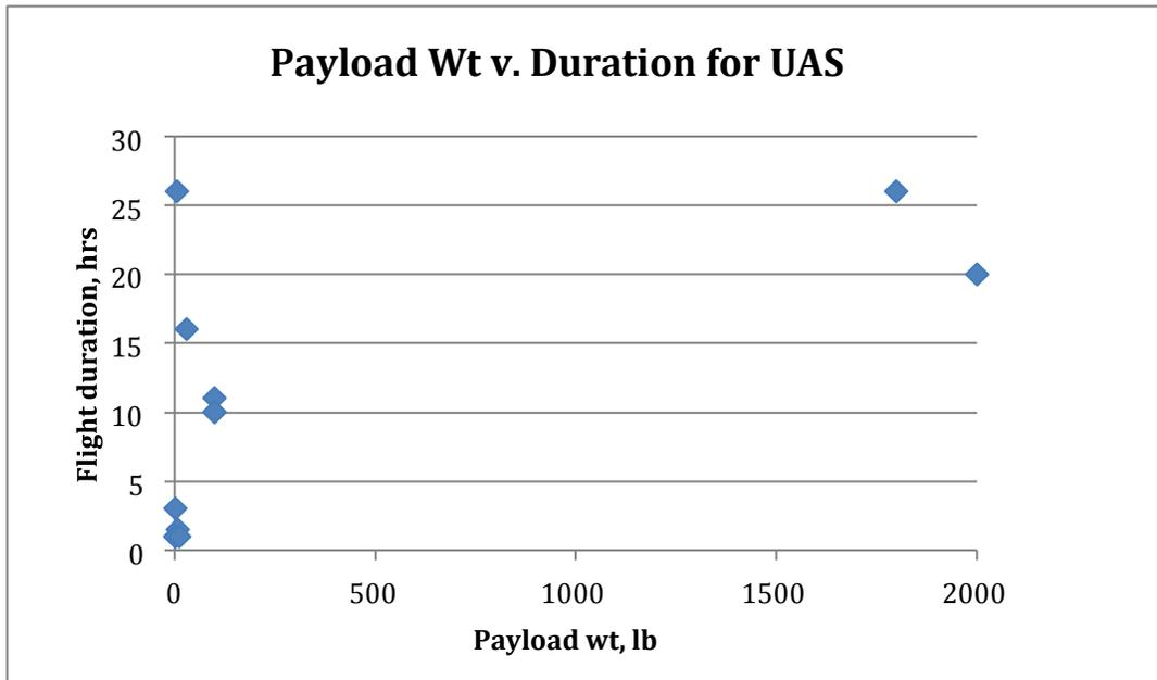
*Figure 7. Payload / flight duration regime of current UAS*
