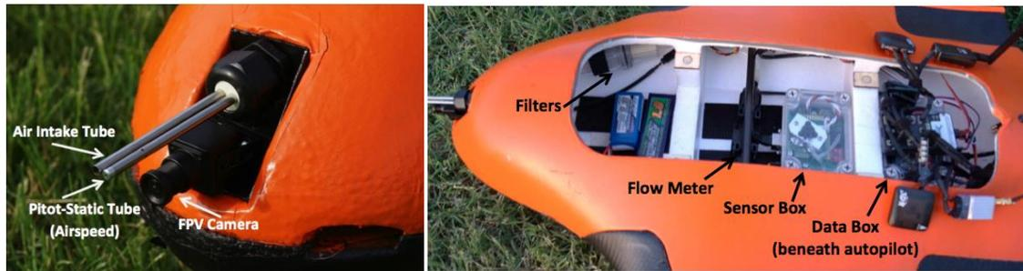
**Figure 9.** Sample gas sensing system with integrated environmental sensors including CO<sub>2</sub> & CH<sub>4</sub>.
