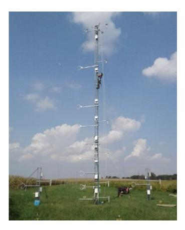
ISFS uses the NCAR In-situ Data Acquisition Software (NIDAS) to provide data ingest, archival, and display. ISFS integrates data from both network and intensive modes with a common data ingest, archival, and display system. Solar power, cellular modems, and satellite data transmission provide the necessary flexibility for ISFS to operate in remote areas.
