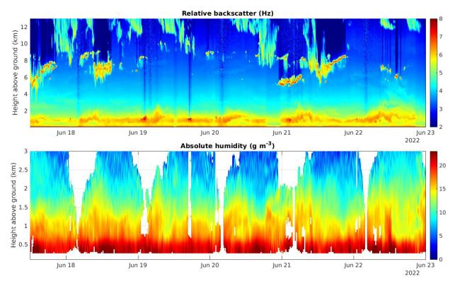
MPD data collected in June 2022 during the Taiwan-based PRECIP field program. The top panel shows relative backscatter; the bottom panel shows absolute humidity.
