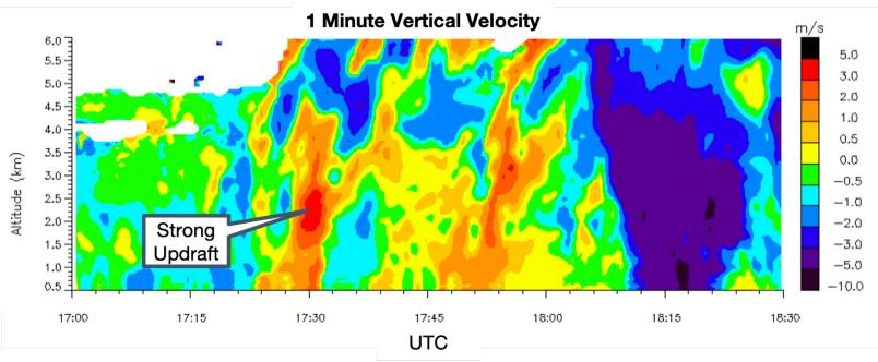
The data plot shows 1 min vertical velocity data from the NCAR 449 MHz wind profiler (3 panels) during the CHEESEHEAD campaign in summer 2016.
