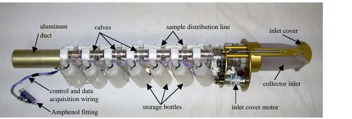
$D_{50}$ =8 µm This size was chosen to collect most cloud drops but exclude smaller, unactivated aerosol particles.
