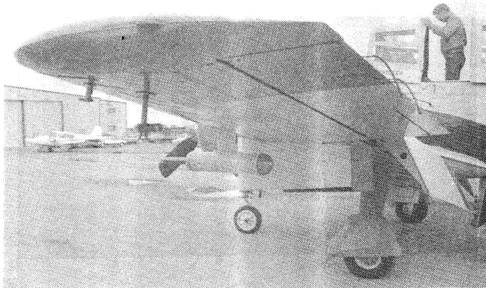
The T-28 is shown from its left side. The instrumentation on its left reverse-flow temperature probe, a PMS Forward Scattering Spectrometer Probe, and a hail spectrometer. A rotating-vane electric field mill is visible on the baggage compartment door which is open and hanging below the fuselage just aft of the wing. [This photo does not show the wing-tip field mill which was installed later.]
