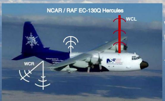
WCL: 1 beam— vertical up no blind zone, nearest ~100 m corrected for overlap ~3.75 m along-beam sampling
