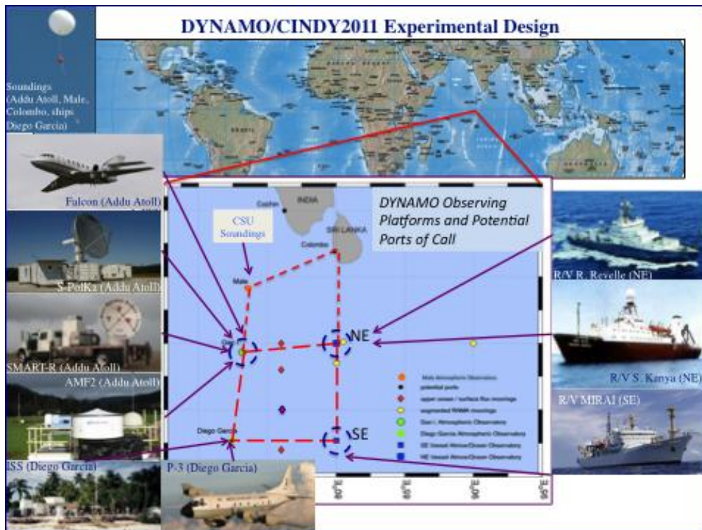
Figure 1. DYNAMO observing facilities deployment in the central Indian Ocean. Ships aircraft and ground based radars, profilers and sounding systems as well as ocean moorings and buoys were spread across the region to measure the MJO as it formed and moved across the region.
