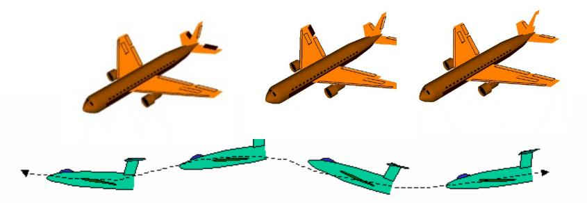
The phugoid frequency for low-damped airplanes ~ sqrt(2) g/( $2\pi$  U) =0.01 Hz.
