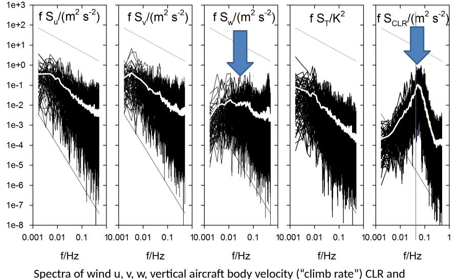
temperature T data vs. frequency f. From 153 constant-level flight legs, 10 min each.
