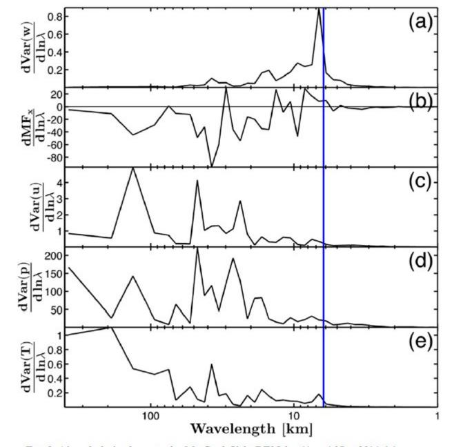
FIG. 9. Aircraft-derived spectra for Mt. Cook flight RF05, leg 11 on 16 Jun 2014: (a) w power, (b) MFx, (c) u power, (d) p power, and (e) T power. The vertical blue line is the estimated buoyancy cutoff for this leg. Note the shift in dominant wavelength between (a) and (c)–(e).
