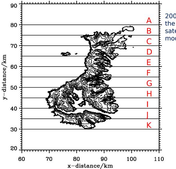
200 m horizontal resolution from the ASTER (on NASA's Terra satellite) global digital elevation model
