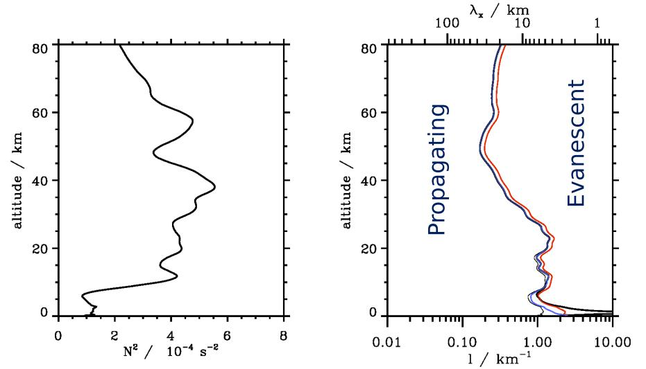
**thick black line**: u **red line**:  $u_{ROT1}$  (magnitude of positive  $u_{\parallel}$  and  $v_{\parallel}$  with 300° along track direction thin black line:  $v_{H}$  **blue line**:  $u_{ROT2}$  (wind direction turns from 320° to 270° in the lowest 10 km)
