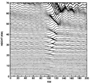
FIG. 2. Particle displacements associated with mountain waves are shown at different altitudes. The mountain is centered at 100 km and is profiled by the lowest displacement line. Panel (a), shows results using the winter wind profile; panel (b), the equinox wind profile. Shaded regions indicate zones where Ri < 1/4.
