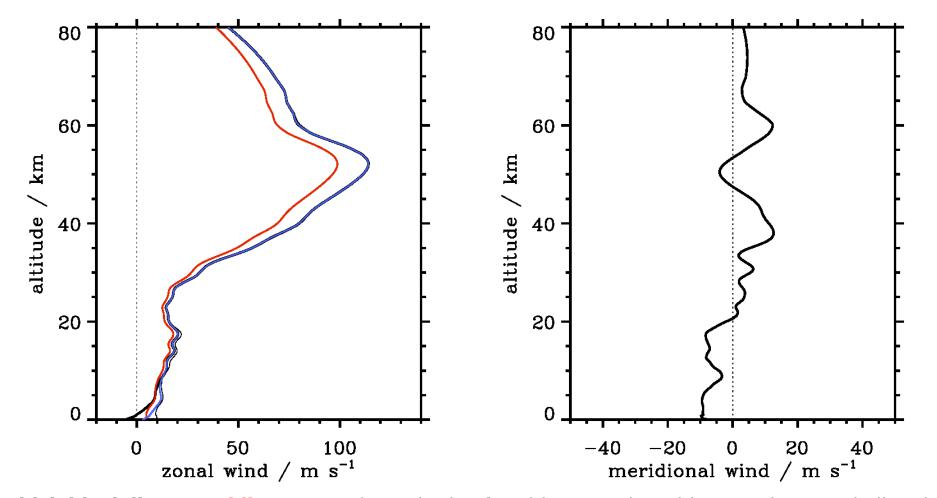
**thick black line**: u **red line**:  $u_{ROT1}$  (magnitude of positive  $u_{\parallel}$  and  $v_{\parallel}$  with 300° along track direction thin black line:  $v_{H}$  **blue line**:  $u_{ROT2}$  (wind direction turns from 320° to 270° in the lowest 10 km)
