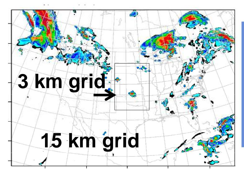
3 km grid configuration Morrison cloud physics MYJ PBL scheme MOZART gas chemistry GOCART aerosol scheme No lightning NO<sub>x</sub> sources
