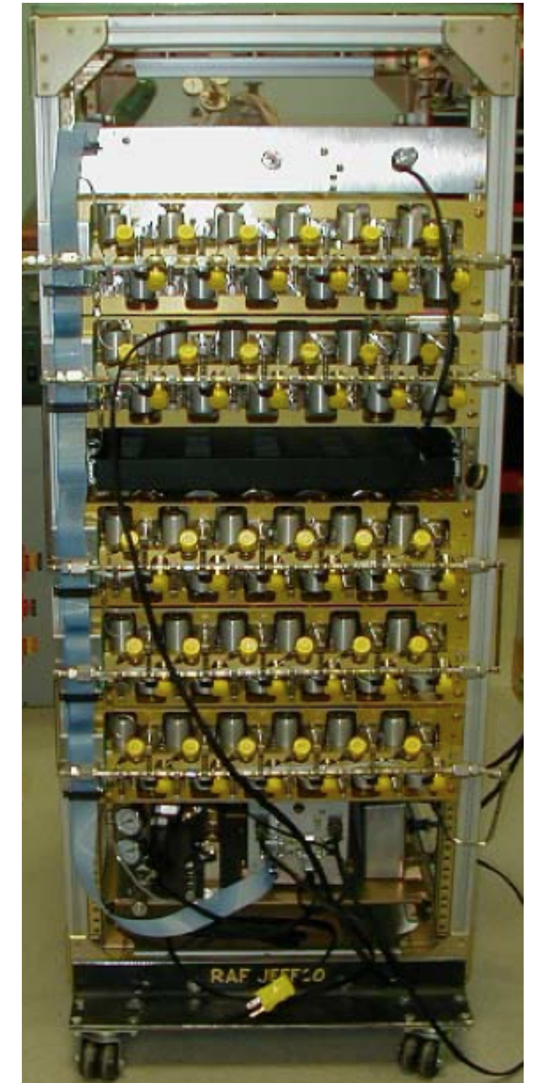
HAIS Advanced Whole Air Sampler (AWAS) during laboratory tests. Bottom rack holds pump, electronics, and pneumatics for sample valves.
