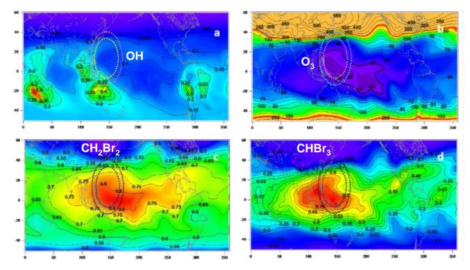
Calculated distributions, CAM-CHEM, for January at 200 hPa. Concentric ovals indicate range of GV aircraft for a 6 hr flight and 8 hr flight, respectively.
