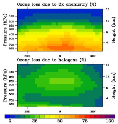
Fig. 6. Percentage of the annually integrated chemical ozone loss from  $HO_x$ ,  $O_x$  and halogen photochemistry as simulated by CAM-Chem.
